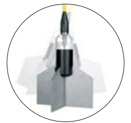
The Current Sensor angles like a pendulum when exposed to currents. The angle is measured and converted electronically to cm/sec.
