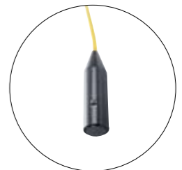
The absolute oxygen concentration is measured by illuminating a membrane with modulated blue light and by reading the phase changes in the reflected red light. The signal is then linearised and temperature compensated.
