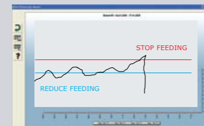
The sensor regulates the feeding based on amount of uneaten pellets passing the sensing area of the Doppler DPS.
