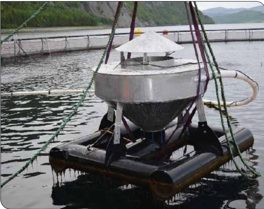
Illustration 5: Lifting the AKVA Subsea Feeder
