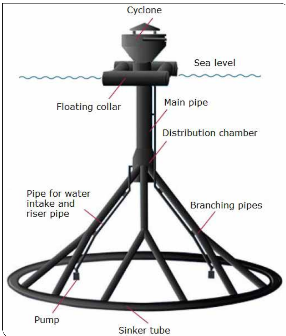
Illustration 1: AKVA Subsea Feeder components
