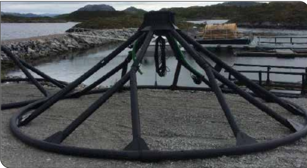
Illustration 3: Properly stored AKVA Subsea Feeder bottom part.
