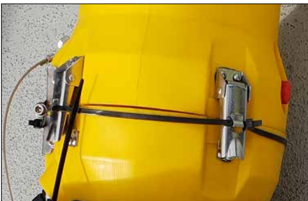
Illustration 16: Place plastic strips around the eccentric locks
