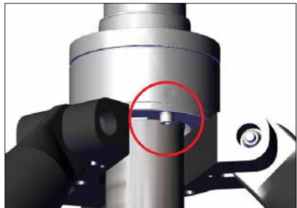
Illustration 31: Base feeding pipe passage bolts
