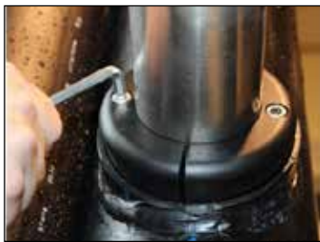
Illustration 14: Attach the tie bolts (9)
