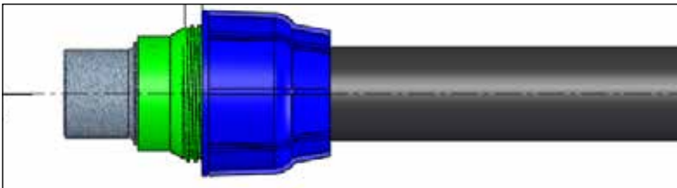
Illustration 22: Feeding pipe connector parts, Union
