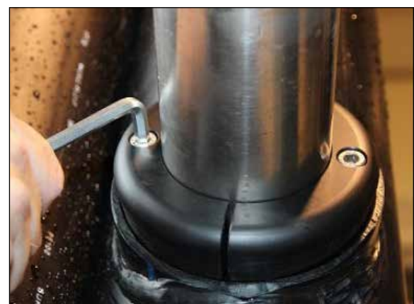
Illustration 31: Base feeding pipe passage bolts
