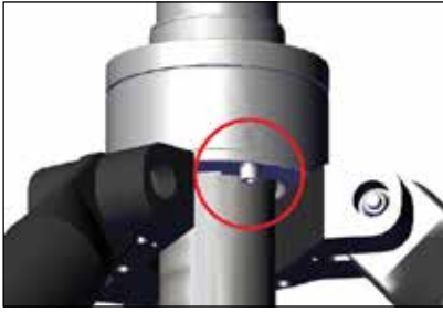
Illustration 13: Place and attach bearing to bearing plate
