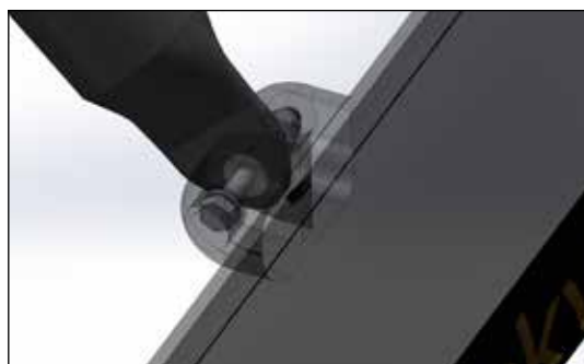
Illustration 3: New reinforcing metal sleeve
