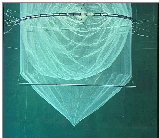
Model testing - Canada treatment sweepnet
