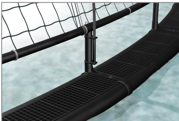
Bird net pole fitted to round handrail support
