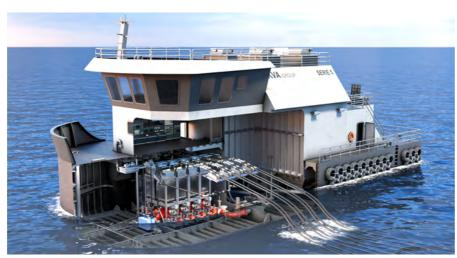
Figure 24 - Barge with waterborne feeding system
